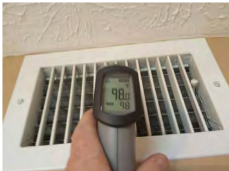
Heat cycl being tested.
